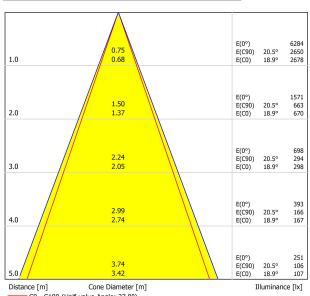
Distance [m] Cone Diameter [m C0 - C180 (Half-value Angle: 37.8°) C90 - C270 (Half-value Angle: 41.0°)
